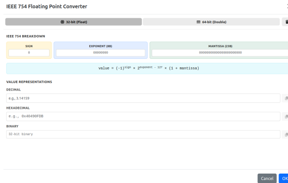
Figure 40: Calculator/converter IEEE 754 of decimal, hexadecimal, simple, and double precision values .
